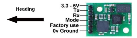
To use the serial mode of operation the mode pin must be connected to ground.
