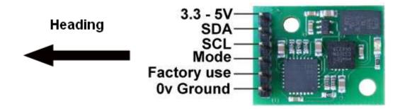
To enter the I2C mode of operation leave the mode pin unconnected
