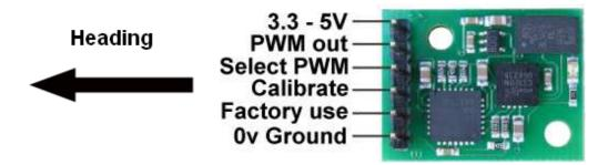
To enter the PWM mode of operation you are required to connect the Select PWM pin to ground. After 500ms the module will enter PWM mode and output a variable high pulse from the PWM out pin dependant on the angle of the PCB.
