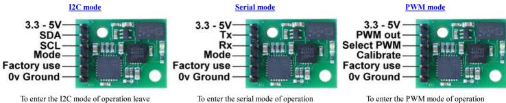
To enter the serial mode of operation connect the mode pin to ground To enter the PWM mode of operation connect the select PWM pin to ground
